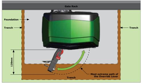
FIGURE 10. MINIMUM CLEARANCES - FRONT
