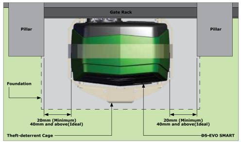
FIGURE 9. MINIMUM CLEARANCES - SIDES
