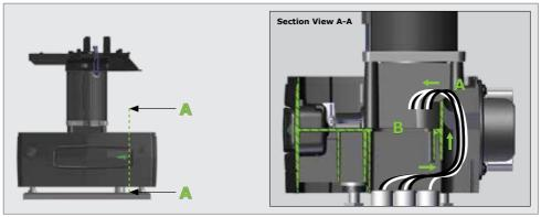
FIGURE 43. CABLE ROUTING FOR RETRO-FITS WITH LONGER CABLES
