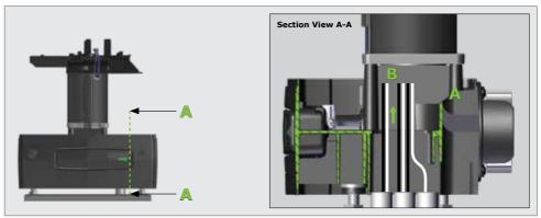
FIGURE 44. CABLE ROUTING FOR RETRO-FITS WITH SHORTER CABLES
