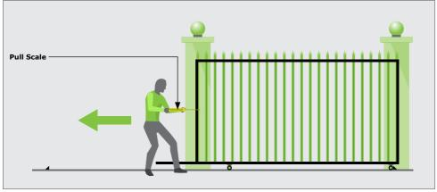
FIGURE 6. STARTING AND RUNNING FORCES
