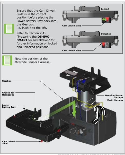
FIGURE 72. LOWER BATTERY TRAY PLACEMENT
