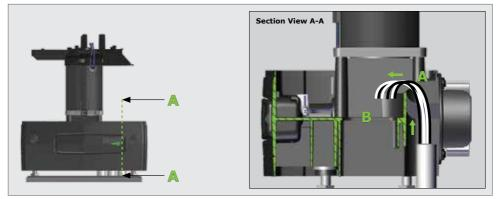
FIGURE 42. CABLE ROUTING FOR NEW INSTALLATIONS
